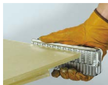
Work horizontally to collect dust
